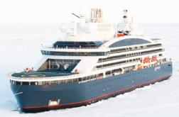
LE COMMANDONT CHARCOT is the first deep polar expedition cruise ship to be equipped with a hybrid liquefield natural gas (currently the cleanest energy available) propulsion and a bank of high capacity batteries
